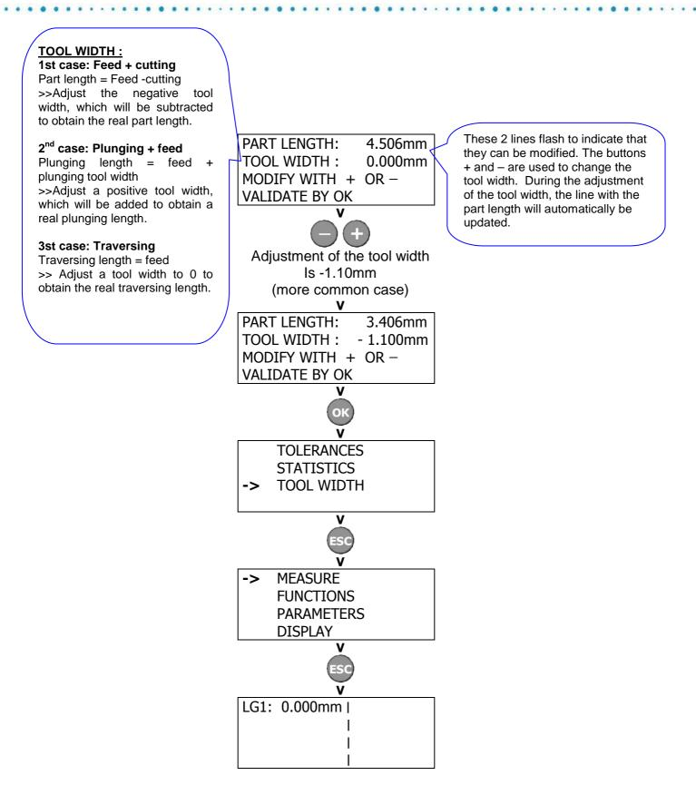
The tool width is adjusted. Now the tolerance should be set.
