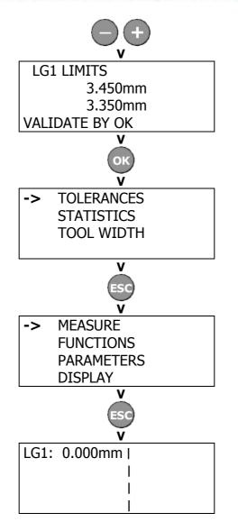
The tolerance limits are adjusted. The gauge is ready to work.
