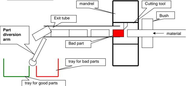
The bad part must pass through the exit tube before it can be isolated from the good parts. The number of parts in the tube can change and this can make the sorting uncertain at the end of the tube.
